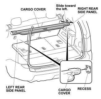
5. Slide and hitch the right and left hooks of the cargo cover to the right and left rear side panel.
