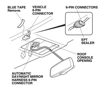
12. Wrap the EPT sealer onto the joint of the 6-pin connectors.
