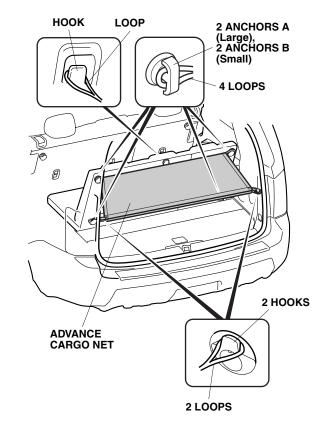
23. Attach two loops on the advance cargo net to two hooks.
