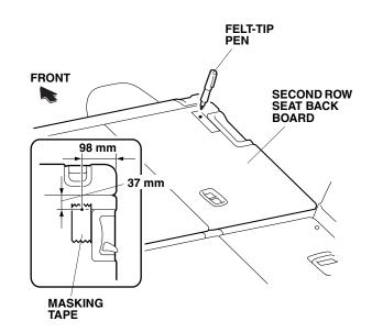
12. Using a felt-tip pen, measure and mark on the masking tape attached in step 10.
