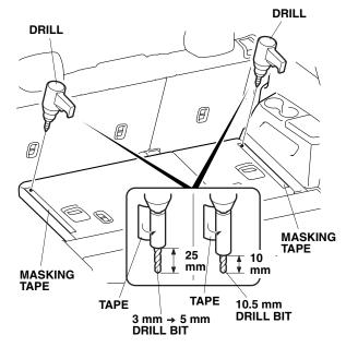
7. Drill at the marked location with a 10.5 mm drill bit. To drill through the hard board only, wrap tape around the drill bit 10 mm away from the tip as shown. 8. While wearing eye protection, drill at the marked locations with a 3 mm drill bit and then with a 5 mm drill bit then drill the hard board and sheet metal. To prevent damage to the inner vehicle parts, wrap tape around the drill bit 25 mm away from the tip to the root as shown.
