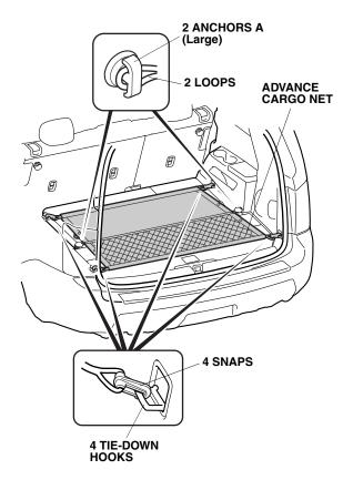
26. Attach four snaps on the advance cargo net to four tie-down hooks and two loops on the advance cargo net to two anchors A (Large) on the third row seat back board.
