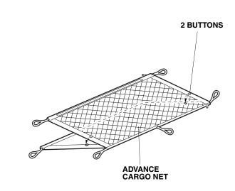
22. Attach five loops on the advance cargo net to two anchors A (Large), two anchors B (Small) and hook on the third row seat back board.
