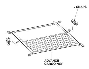
28. Attach four loops on the advance cargo net to two hooks and two anchors B (Small) on the third row seat back board.
