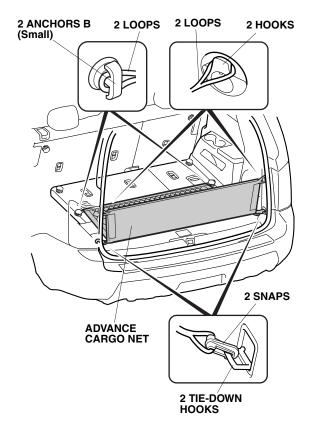
29. Attach two snaps on the advance cargo net to two tie-down hooks.
