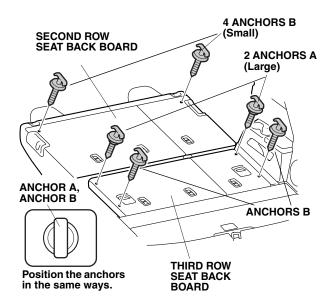
Install the four anchors B (Small) on the second and third row seat back board into the holes made in step 8 and 13.
