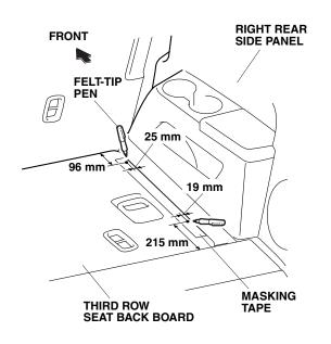
5. Using a felt-tip pen, measure and mark two locations on the masking tape attached in step 3.
