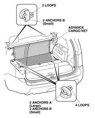
20. Attach six loops on the advance cargo net to two anchors A (Large) and four anchors B (Small) on the second and third row seat back board.
