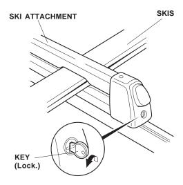
With the skis attached, rock the attachment in all directions to make sure it is installed securely. Adjust as necessary.
