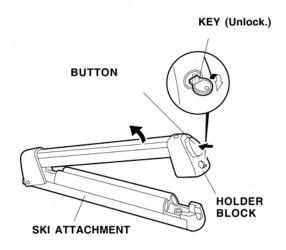
Position the skis on the attachment with the rear of the skis facing forward, and the bindings between the front and rear attachments.
