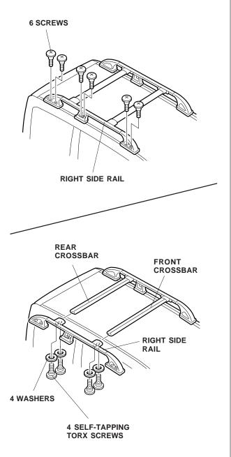
Remove the rubber moldings from the front and rear roof rack crossbars. Retain the rubber moldings to reinstall later.
