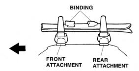
If both bindings cannot be positioned between the front and rear attachments, install the skis with one of the bindings positioned behind the rear attachment.
