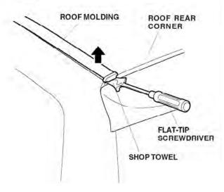
Remove the roof moldings by carefully lifting them upward.
