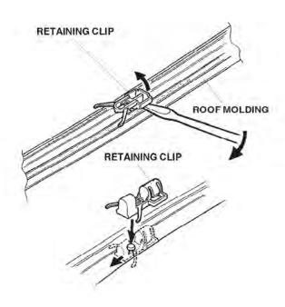
If any of the six center retaining clips remained on the roof, remove them from the stud bolts using long nose pliers.
