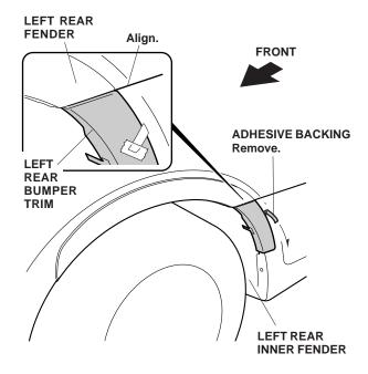
12. Using a rubber roller, apply pressure against the fender trim and roll from one end to the other.
