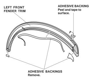
Using an alcohol swab, throughly clean the area where the left front fender trim will attach. Align the tip of the left front fender trim with the edge of the masking tape as shown.
