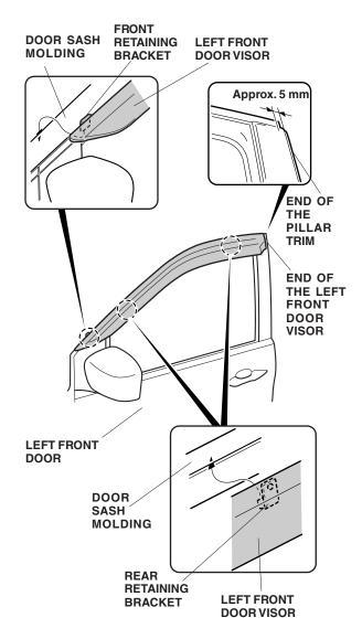
5. Hook the front retaining bracket into the door sash; push two rear retaining brackets into the door sash molding.
