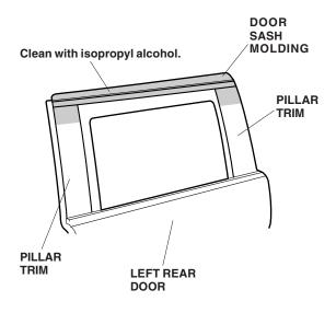
11. On the back of the left rear door visor, peel back 1 to 1 1/2 inches (26–38 mm) of the adhesive backings, and tape them to the front surface of the left rear door visor with a masking tape.
