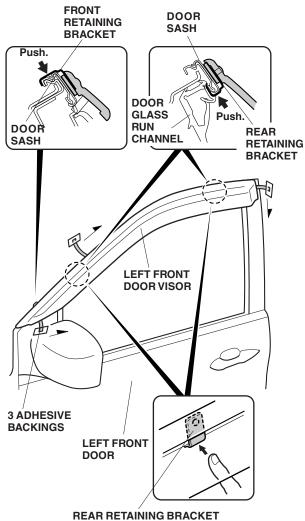
REAR RETAINING BRACKET Press on the door visor firmly while removing the adhesive backings.
