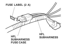
13. Plug the HFL subharness 6-pin connector into the 6-pin opening in the fuse box.
