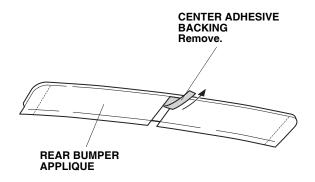
3. Place the rear bumper applique on the rear bumper, and align the cutout with the tailgate latch anchor as shown.
