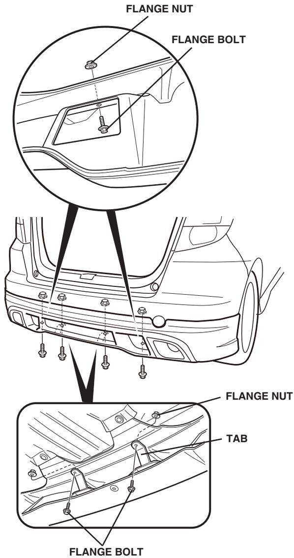
24. Install the outboard bumper clips through the under spoiler brackets. Be sure to install the rubber washer between the bracket and the splash shield on the driver's side of the vehicle.
