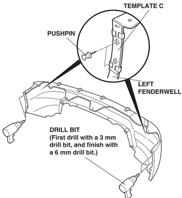
11. While wearing eye protection, drill the pierced marks on the bumper.
