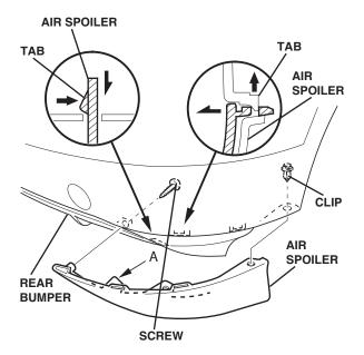
4. Place template A on the rear bumper as shown, and mark the height of the rear under spoiler with a white marker.
