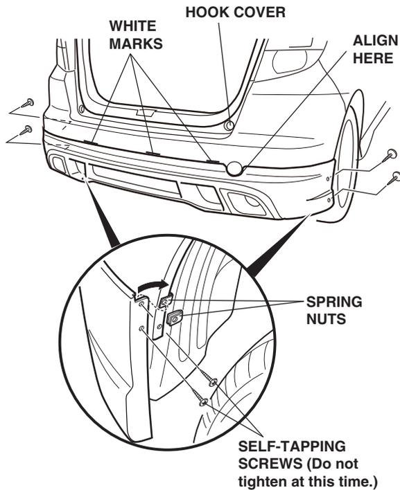
17. Install the four self-tapping screws, and the four spring nuts (two on each side). Do not tighten the self-tapping screws at this time.
