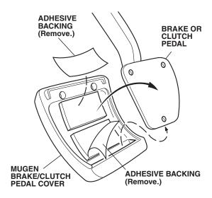
9. Remove the adhesive backing from the Mugen brake pedal cover. Align the top of the brake pedal cover over the brake pedal as shown, and press the pedal cover into position.
