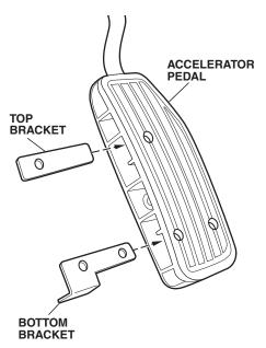
5. Place the Mugen accelerator pedal cover on the accelerator pedal with the top edge and the side edge of the rubber spacer tight against the pedal. Insert the three rivets through the pedal, the brackets, and the pedal cover at the holes shown.
