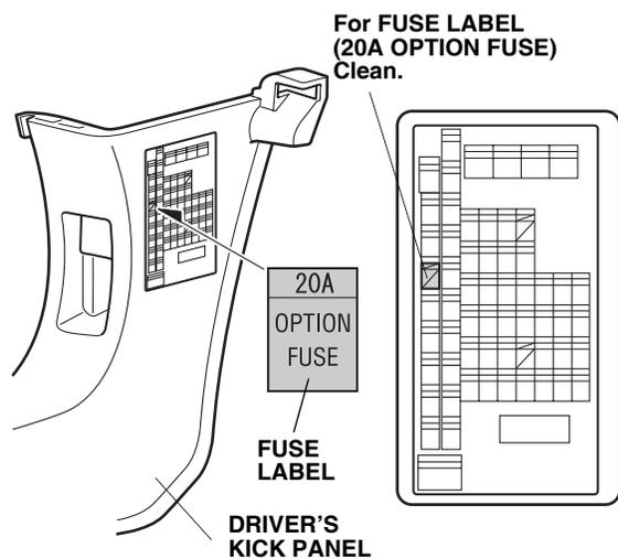
24. Attach the fuse label (20A OPTION FUSE) to driver's kick panel as shown.
