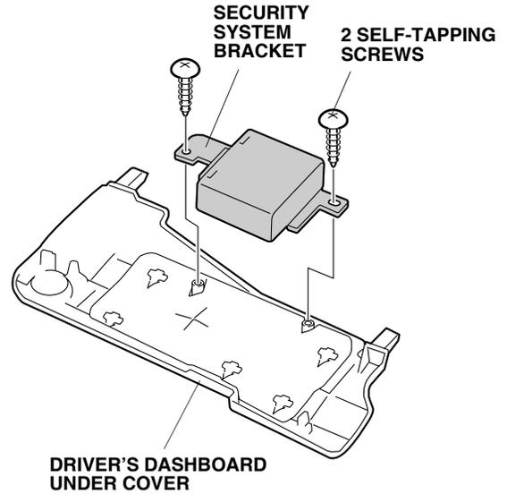
22. Plug the security system harness 18-pin connector to the control unit. Reinstall the driver's dashboard under cover.
