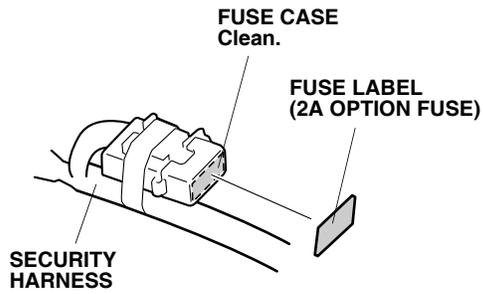
11. Attach the fuse label (2A OPTION FUSE) to the security system harness fuse case.
