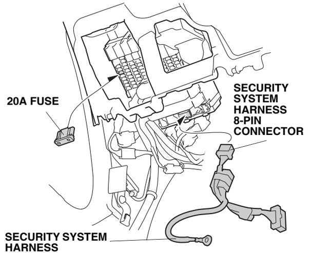
13. Install the 20A fuse to the fuse box in the location shown.
