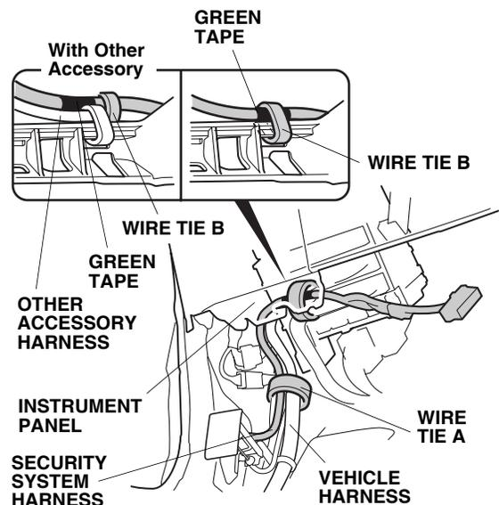
18. Using one wire tie B, secure the security system harness to the instrument panel as shown. If the vehicle is equipped with another accessory, use one wire tie B to secure the security system harness to the other accessory harness.
