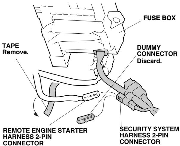
15. Remove the dummy connector from the security system harness 2-pin connector and plug the remote control engine starter harness 2-pin connector to the security system harness 2-pin connector.
