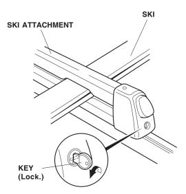
With the skis attached, rock the attachment in all directions to make sure it is installed securely. Adjust as necessary.
