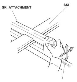
Rock the ski attachment in all directions to make sure it is installed securely.
