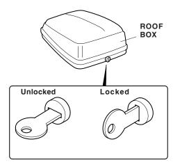
**Locking**: Press down on the lid. You should hear an audible click. Be sure the lid is latched by attempting to lift the lid. Turn the key clockwise to lock the roof box. Remove the key while not in use. Be sure the straps are not outside of the roof box.
