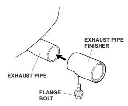
2. With the flange bolt facing down, slide the exhaust pipe finisher onto the exhaust pipe until it bottoms.
