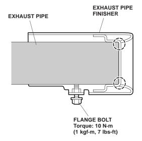
4. Start the engine and rev it up a few times. Listen for vibration from the exhaust pipe finisher and adjust if necessary.
