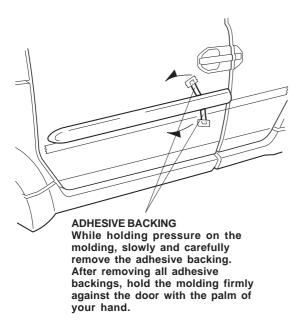
6. Using a hard rubber roller, roll the long body side molding from one end to the other.
