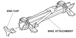
Turn and loosen the mounting levers on the bike attachment.
