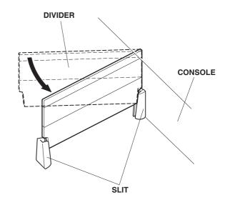
3. Check that the divider is set in both slits of the console and push the divider down to install it in the slits securely.
