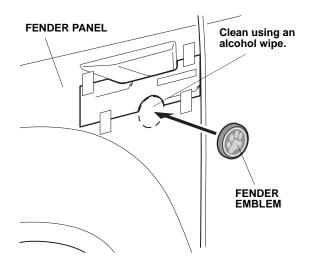
10. Place the fender emblem on the fender panel and align top edge of the emblem with the lower edge of the fender template.
