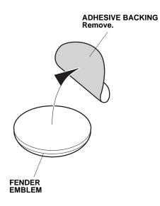
9. Using an alcohol wipe, thoroughly clean the area where the fender emblem will attach.
