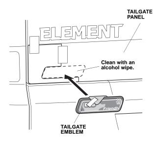
4. Place the tailgate emblem on the tailgate panel, and fit the emblem into the template as shown.
