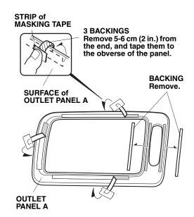
8. Attach the strip of masking tape to the end of each shaded backing. Peel back 5-6 cm (2 in.) of the backings and fold them over as shown. Temporarily attach the strips of masking tape to the obverse of the outlet panel A. Remove all remaining backings from the outlet panel A.
