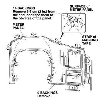
Attach a strip of masking tape to the end of each shaded backing. Peel back 5-6 cm (2 in.) of the backings and fold them over as shown. Temporarily attach the strips of masking tape to the obverse of the meter panel. Remove all remaining backings from the meter panel. Position the meter panel on the existing meter panel.
