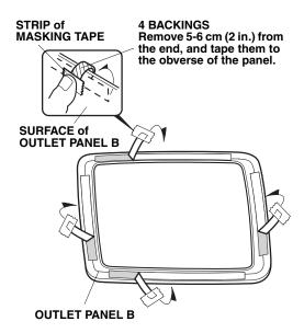
10. Position the outlet panels A and B on the existing outlet panels. While holding pressure on the outlet panels, carefully remove the backings from the outlet panels. Hold the outlet panels A and B firmly against the existing outlet panels with the palm of your hand, particularly at the edges.
