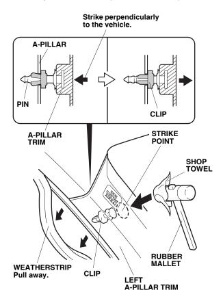
15. Using a rubber mallet and a shop towel, lightly tap the left A-pillar trim just below the "SIDE CURTAIN AIRBAG" mark to release the clip.
