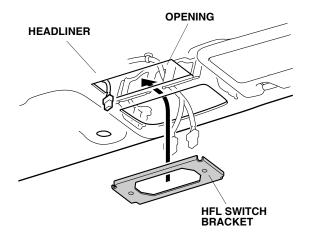
48. Route the HFL harness out the headliner opening, and plug the white 20-pin connector into the switch. Secure the switch to the HFL bracket with two 5 x 12 mm pan screws.
