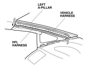
27. Loosely secure the HFL harness to the vehicle harness with four wire ties. If the vehicle is equipped with the washer tube, do not secure the wire ties around the washer tube.
