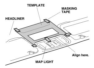
5. Measure 145 mm from the front edge of the headliner and align the template to the headliner as shown. Tape the template to the headliner with masking tape.
