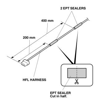
29. Route the HFL harness to the opening in the headliner, and leave 80 mm of the HFL harness extending from the opening.
