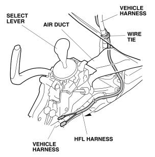
39. Secure the HFL harness to the vehicle harness with one wire tie.
