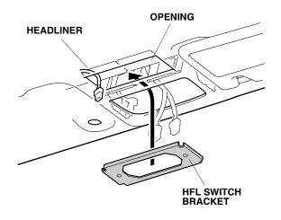
45. Route the HFL harness out the headliner opening, and plug the white 20-pin connector into the switch. Secure the switch to the HFL bracket with two 5 x 12 mm pan screws. Go to step 49.
