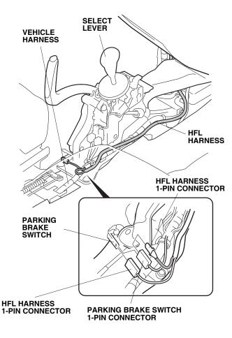
41. Secure the HFL harness to the vehicle harness with three wire ties. Do not secure the wire ties to the SRS harness.
