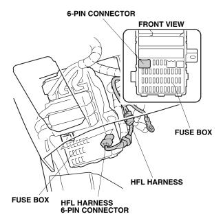
If another harness is already plugged to the fuse box, unplug it. Remove the dummy connector from the HFL harness 6-pin connector taped to the HFL harness, and plug the other accessory 6-pin connector into the HFL harness. Plug the HFL 6-pin connector into the fuse box.
