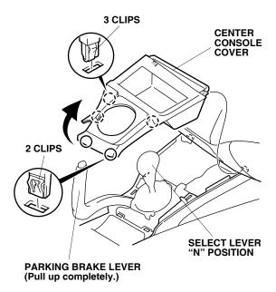
19. Open the center console lid, and remove the mat.
