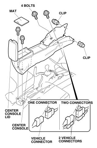
Remove the center console (four bolts, two clips, and unplug one vehicle connector or two vehicle connectors). 21. If equipped, remove the driver's under cover (turn the knob counterclockwise, two clips and one pin).
