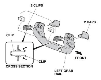
59. Reinstall the left grab rail with two clips and two caps.
