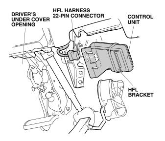
55. Secure the HFL bracket to the vehicle bracket with two 6 x 12 mm flange bolts.
