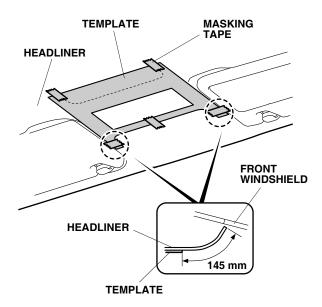
6. Using a felt-tip pen, mark the headliner along the template as shown. Remove the template.
