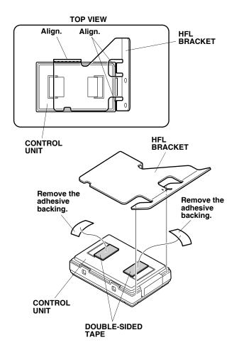
52. Remove two adhesive backings from the control unit and attach the HFL bracket to the control unit.
