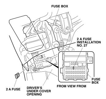
57. Attach the 2 A fuse label to No. 27 slot on the left kick panel.
