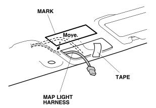
13. Using an utility knife, cut out the headliner at the mark made in step 6.
