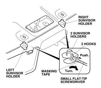
Remove the cover from the left sunvisor (four retaining tabs). Remove the left sunvisor (two T-25 Torx screws, and unplug the vehicle connectors, if equipped).
