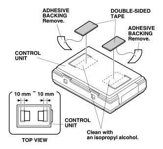
50. Remove the adhesive backings from each double-sided tape and attach the tape to the control unit as shown.
