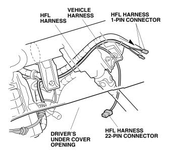
Secure the HFL harness to the vehicle harness with two wire ties.
