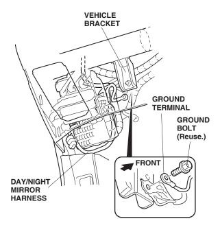
31. Secure the day/night mirror harness to the vehicle harness with four wire ties in the areas shown.
