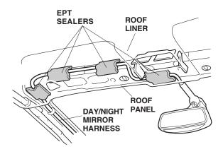
28. Secure the day/night mirror harness to the vehicle harness with three wire ties in the areas shown.
