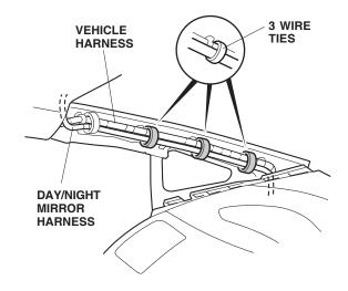
29. Plug the day/night mirror harness 6-pin connector into the 6-pin connector at the fuse box.
