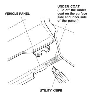
23. Apply touch-up paint to the vehicle panel in the area where you filed off the under coat. Do not install the under bracket until the touch-up paint is dry.
