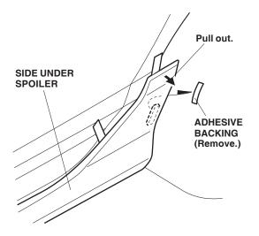
29. Remove the three adhesive tapes from the left side under spoiler. Press on the adhesive part of the side under spoiler firmly.
