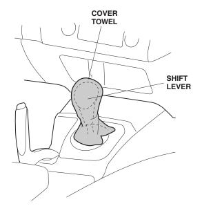
Remove the lid from the dashboard center lower cover (four retaining tabs).
