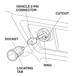
cutout in the ring, and slide the socket into the ring.
