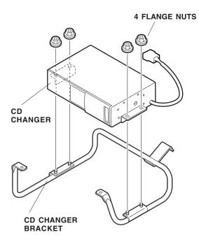
33. Wrap one EPT sealer around the bus cable connector from the CD changer, then secure the bus cable and connector to the CD changer bracket with two wire ties.
