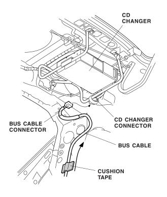
38. Fold the excess bus cable, and secure it to the holes in the rear seat panel with the two wire ties with clip.
