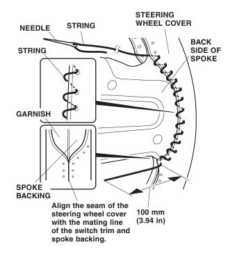
8. After lacing the string through the holes in the steering wheel cover at the back side of the spoke, lace up the steering wheel cover tightly as it wrinkles a little at the end. Best fitment results are obtained by lacing up the steering wheel cover tightly.
