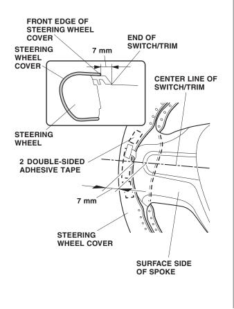
Align the rear edge of the steering wheel cover to the back of the steering wheel spoke as shown. Attach the steering wheel cover to the steering wheel with the double-sided adhesive tape.
