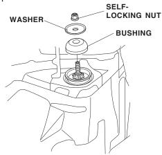
36. Torque the damper shaft self-locking nut to 29 N⋅m (21lb-ft) while holding the damper shaft with a hex wrench.
