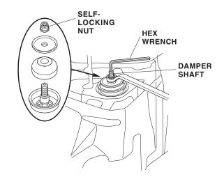
25. Compress the damper unit by hand, and remove it from the vehicle.
