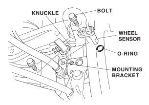
20. Remove the brake hose mounting bracket.
