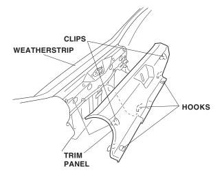
• Remove the clips, then remove the trunk side trim panel. Release the wire harness from the slit in the trim panel.
