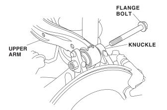
32. Install the damper mounting bushing onto the damper unit, and install the damper unit. Slowly raise the jack until you can align the bolt hole with the holes in the trailing arm and the damper, then install the new flange bolt.
