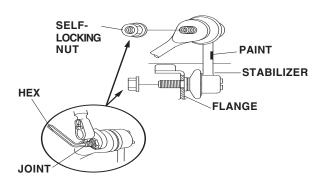
22. Remove the flange bolt that connects the knuckle and the upper arm.
