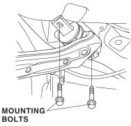
31. Loosely install a new flange bolt on the knuckle and the upper arm.
