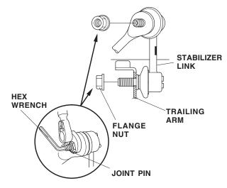
34. Install the stabilizer link on the trailing arm with a new self-locking nut, and lightly tighten both nuts.
