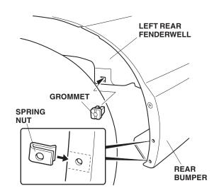
Position the left rear splash guard on the left rear fenderwell and rear bumper, then install the two 5 x 25 mm self-tapping screws and one 5 x 20 mm self-tapping screw. Tighten the three self-tapping screws in the order shown cut off any excessive undercoat material with a utility knife.
