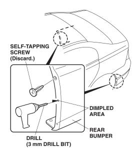
3. Remove and discard the two self-tapping screws from the fenderwell area of the rear bumper.
