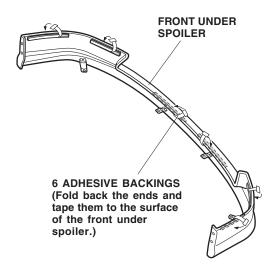
8. Using isopropyl alcohol on a shop towel, clean the front bumper where the front under spoiler will attach.
