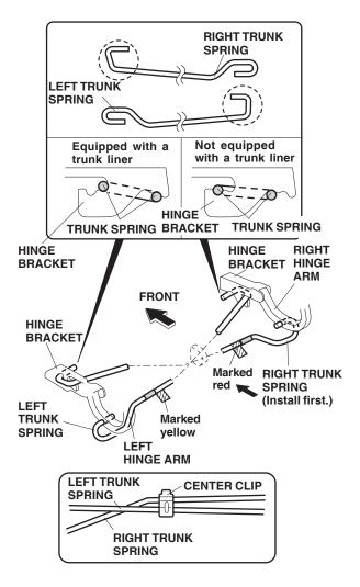
6. Reinstall the center clip on the trunk springs.
