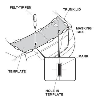
11. Position the template A on the trunk lid. Using a felt-tip pen, mark the trunk lid on the left and right sides.
