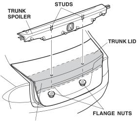
Thoroughly clean the surface where the trunk spoiler will be attached with isopropyl alcohol.
