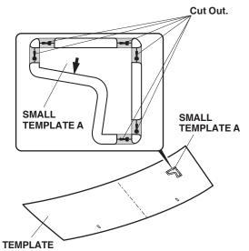
10. Align the front edge of the template with the front edge of the trunk lid. Center the template from side to side. Secure the template with tape. Using a felt-tip pen, mark the two places on the trunk lid. Remove the template.
