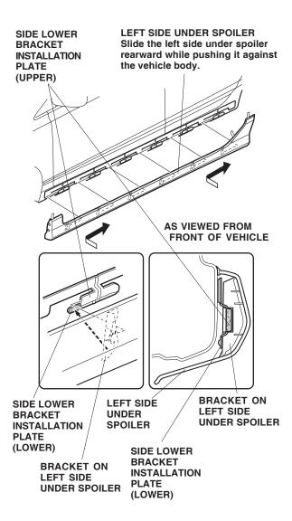
20. Check that all six brackets of the left side under spoiler are set in the side lower bracket installation plates. Check that there is no excessive gap between the left under spoiler and the vehicle. If an excessive gap is found, repeat step 19.
