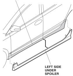
2. Using a tape measure and felt-tip pen, measure and mark the body area shown.
