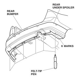
NOTE: If a gap is visible between the rear bumper and under spoiler, remove the under spoiler and confirm the locations of the marks with a tape measure. If necessary, create new marks in the proper locations.
