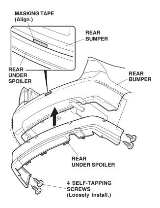
8. While applying pressure to the rear under spoiler, use a felt-tip pen to mark the rear bumper at each hole in the bracket on the rear under spoiler.
