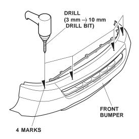
While wearing eye protection, drill a 3 mm hole through each of the four dimples on the ends of the front bumper. Remove any burrs from the edges of the holes with a file.
