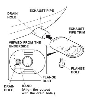
Slide the exhaust pipe trim onto the exhaust pipe until it bottoms against the exhaust pipe.
