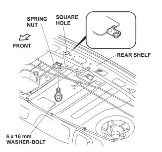
15. Loosely install a 6 x 16 mm washer-bolt to the spring nut.
