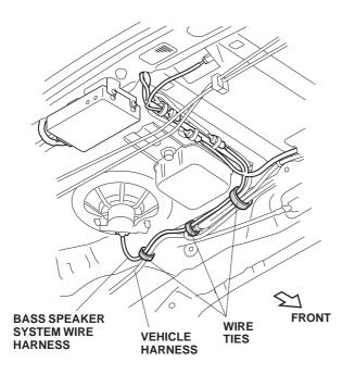
36. Wrap an EPT sealer around each 2-pin connector in the area shown, then secure the bass speaker system wire harness to the vehicle harness with two wire ties over the EPT sealers.
