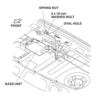
18. Thread the other 6 x 16 mm bolt through the rear shelf and into the threaded bracket.
