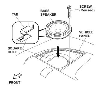
34. Plug the bass speaker system wire harness 2-pin connectors into the right and left bass speakers.
