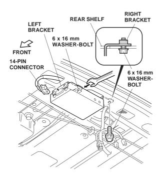
20. Plug the bass speaker system wire harness 14-pin connector into the bass unit.
