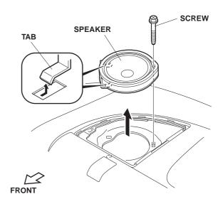
33. Install the right and left bass speakers using the screws removed in step 32.
