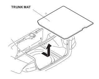
4. Remove the front trunk panel (six clips).
