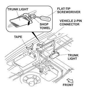
22. Using a flat-tip screwdriver wrapped with a shop towel, remove the trunk light (two tabs), and unplug the vehicle 2-pin connector.
