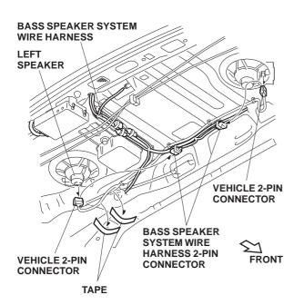
30. Unplug the right and left speaker wires from each speaker, and plug the speaker wire 2-pin connectors (white) into the bass speaker system wire harness 2-pin connectors.
