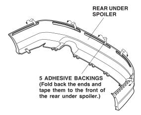
8. Using isopropyl alcohol on a shop towel, clean the rear bumper where the rear under spoiler will attach.
