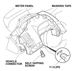
9. Apply masking tape to the instrument panel as shown, and remove the center panel (two bolts and 11 clips, and unplug the vehicle connectors).
