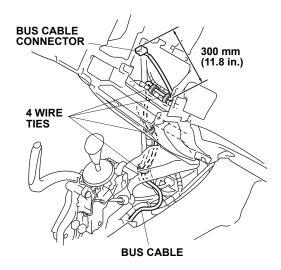
24. Along the center console area, secure the bus cable to the vehicle harness with three wire ties.
