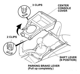
12. Open the center console lid, and remove the mat.
