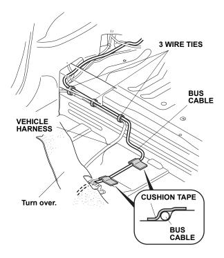
27. Secure the bus cable to the vehicle harness with the three wire ties in the areas shown.
