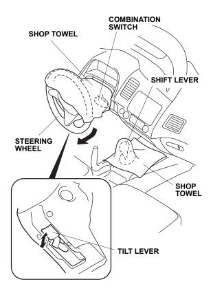
7. To protect the dashboard area, place a shop towel over the steering wheel and shift lever.
