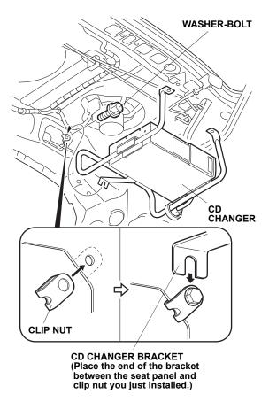
35. Loosely install the washer-bolt to the rear seat panel first. Then, place the end of the CD changer bracket between the seat panel and clip nut you just installed.
