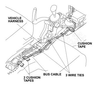
25. Using isopropyl alcohol on a shop towel, clean the areas where the cushion tape will attach. Attach the bus cable to the floor panel with the three cushion tapes in the area shown.
