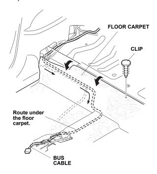
21. Route the bus cable forward to the right front console frame along the vehicle harness.
