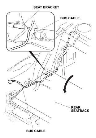
20. Lift up and lock the right rear seat-back, then remove the clip that secures the floor carpet. Pull back the floor carpet. Route the bus cable under the floor carpet as shown.
