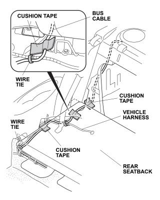
29. Using isopropyl alcohol on a shop towel, clean the areas where the cushion tape will attach. Attach the bus cable to the floor panel with the three cushion tapes in the areas shown.
