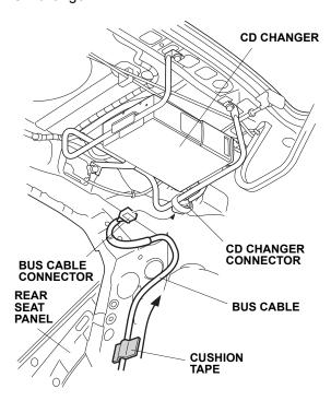
38. Using isopropyl alcohol on a shop towel, clean the area where the cushion tape will attach. Attach the bus cable to the rear seat panel with one cushion tape.
