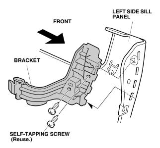
13. Install the bracket to the left running board with one of the screws removed in the above step.
