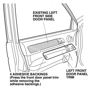
15. Repeat steps 12 thru 14 to install the door panel trims for the remaining three doors.
