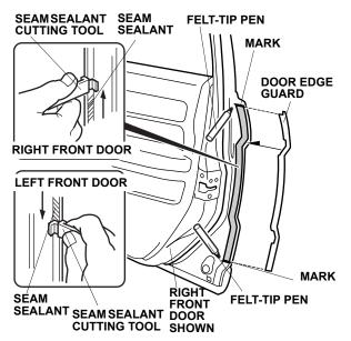
4. Position the cutting edge of the seam sealant cutting tool against the door edge, and trim the seam sealant from mark to mark.
