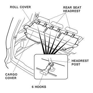
5. Slide both ends of the rear roll cover rod into the recesses in the rear side trim panel.
