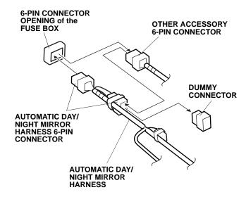
Attach a piece of steel wire to the automatic day/ night mirror harness, and route it through the left front pillar trim opening.
