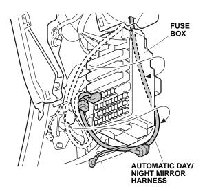
18. Remove the steel wire. Route the automatic day/ night mirror harness along the vehicle harness as shown. Loosely secure the day/night mirror harness to the vehicle harness with the four wire ties.
