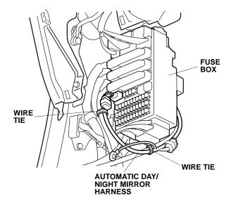
25. Remove the vehicle bolt from the fuel lid opener. Attach the automatic day/night mirror harness ground terminal with the ground bolt supplied.
