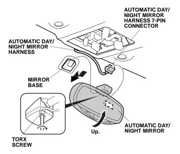
21. Install the day/night mirror on the mirror base, then tighten the T-20 TORX screw installed in the day/night mirror.
