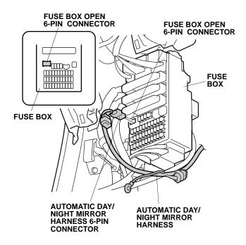
NOTE: If another accessory is already plugged into the 6-pin connector opening of the fuse box, remove the dummy connector from the 6-pin connector taped to the automatic day/night mirror harness. Plug the 6-pin connector from the other accessory harness into the 6-pin connector from the automatic day/night mirror harness you just unplugged and plug the automatic day/night mirror harness into the 6-pin connector opening of the fuse box.
