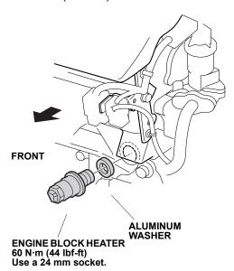
12. Plug the connector end of the heater harness into the engine block heater.
