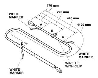
9. Using a white marker, mark the heater harness at the measurements shown.
