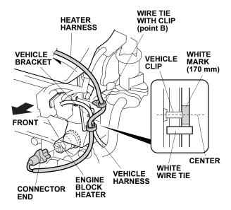
13. Route the heater harness as shown and secure the heater harness to the vehicle harness with one white wire tie at the 170 mm mark you made. Secure the one wire tie with clip (270 mm) to the vehicle bracket.
