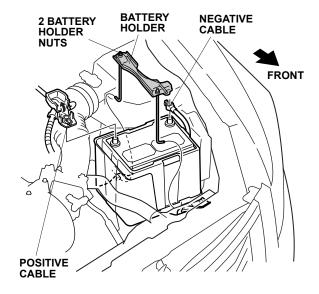
7. Remove the battery cover, battery, and battery box.
