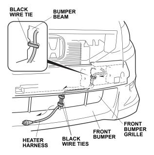
18. Attach the protective cap to the front bumper grille, and plug the heater harness connector into the protective cap.
