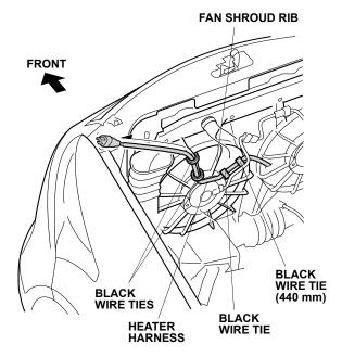
15. Route the heater harness as shown and secure it to the vehicle harness with two black wire ties.
