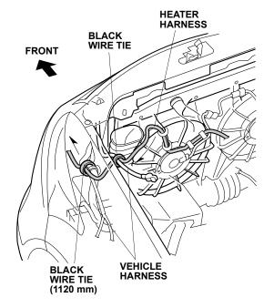
16. Route the heater harness as shown and secure the heater harness to the hole in the vehicle frame with one wire tie with clip.
