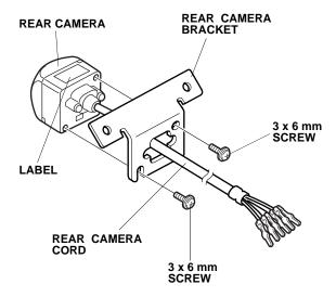
29. Wrap the terminals of the rear camera cord with electrical tape.
