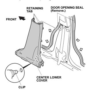
13. Remove the right center lower cover (one clip and four retaining tabs).
