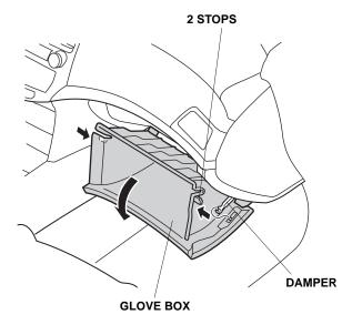
5. Remove the glove box (two screws).
