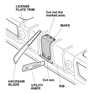
57. Using a utility knife, cut out the rib from the license plate trim as shown.
