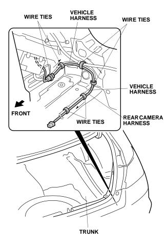
44. Route the rear camera harness forward along the vehicle harness towards the front of the vehicle, and secure it to the vehicle harness with one wire tie.
