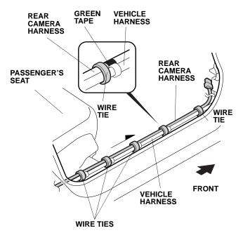
48. Route the rear camera harness up through the glove box opening, and secure it to the vehicle harness with five wire ties.
