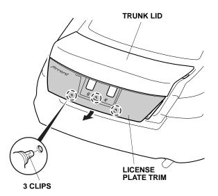
22. Slide the license plate trim down, and disengage the top two clips to remove the license plate trim.
