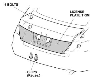
Insert the KTC trim tool (AP201-W) between the license plate trim and the trunk lid. Move the tool left and right to peel off the double-sided tape in between.
