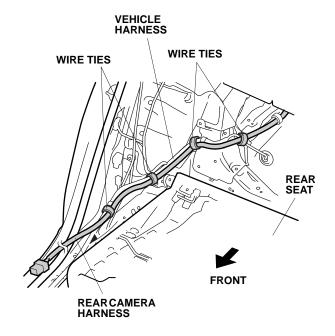
46. Route the rear camera harness forward past the "B" pillar, and secure it to the vehicle harness with three wire ties.
