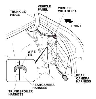
43. Route the rear camera harness along the vehicle harness, and secure it to the vehicle harness with six wire ties.
