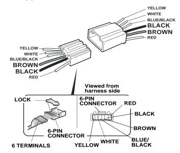
35. Route the rear camera harness through the trunk lid hole, and plug the rear camera cord 6-pin connector into the rear camera harness 6-pin connector.
