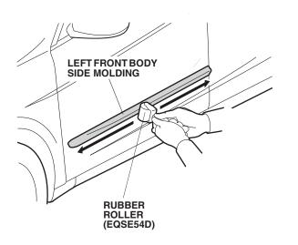
9. Peel back approximately 1 1/2 to 2 inches of the adhesive backing from each adhesive tape, and tape the ends to the outside surface of the body side molding.
