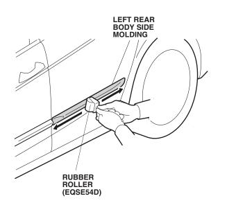
14. Turn the templates over and repeat steps 1 thru 12 to install the body side molding on the right side of the vehicle.
