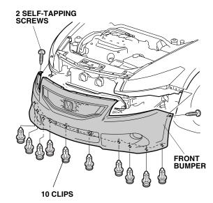
Remove the three self-tapping screws from the front bumper, and remove the left fog light cover or fog light cover/fog light. Remove the right fog light cover the same way.
