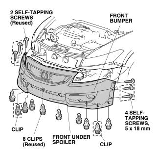
32. While applying pressure on the front under spoiler, carefully remove the adhesive backings starting in the center of the bumper and working outward. After removing, the backings hold the front under spoiler firmly against the front bumper with the palm of your hand for 30 seconds.
