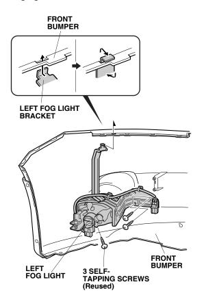
31. Using two self-tapping screws (reused), eight clips (reuse), four 5 x 18 mm self-tapping screws, and two clips, install the front bumper. Reconnect the fog light harness connectors.
