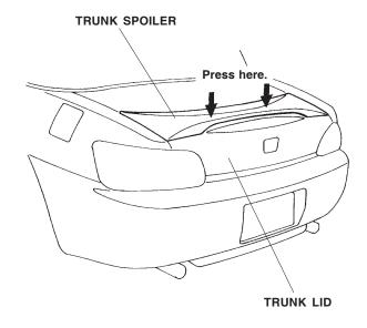
8. Slowly remove the trunk spoiler from the trunk lid. Check that the marking washers stay attached to the trunk lid. 9. Lightly center-punch the trunk lid at the center of each marking washer attached to the trunk lid, then remove the marking washers.
