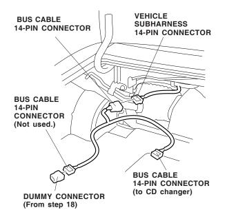
20. Install the dummy connector (from step 18) to the bus cable 14-pin connector.
