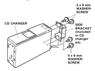
Position the CD changer bracket on the CD changer, and secure the bracket with the six 4 x 8 mm washer-screws.
