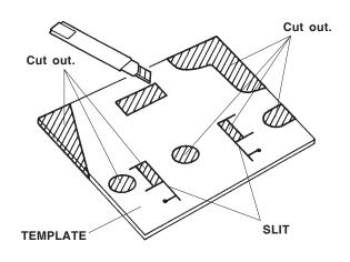
6. Position the template by aligning the round holes in the template with the clip holes, then tape the template in place to the left of the trunk floor trim panel. Mark the edges of the rectangular holes and down along the slit lines on the panel with a felt-tip pen. Make the round marks, and remove the template.
