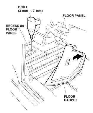
10. Remove the two grommets from the floor panel, and insert the jack nuts into the holes.
