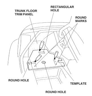
7. While wearing eye protection, lift up the trunk floor trim panel, and drill a 25 mm hole through each of the two marks you made in the panel. Drill the 25 mm holes only through the trunk floor trim panel and not through the trunk floor panel.
