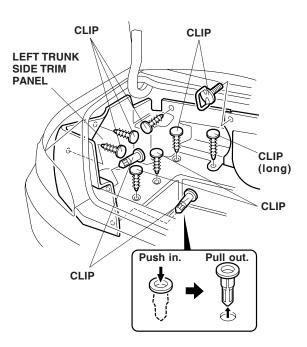
4. Using a tape measure and a felt-tip pen, measure and mark the left trunk side trim panel. Cut out the marked area from the panel with a utility knife.
